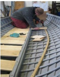
Stringers are now also fitted and the floors currently being manufactured to fit. Getting the floors level was an interesting exercise and here you see a floor stringer being fitted. The thwarts and stern seating have already been made and trial fitted, but await the completion of the floors before final fit.
