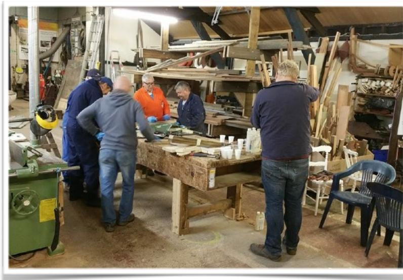
In days gone by internal frames would have been from grown oak which is no longer available. So the team is laminating the frames that will help support the foredeck out of strips of oak pre-bent and then glued together. Engine bearers will be made the same way, but the ribs will be of steamed and bent oak.
